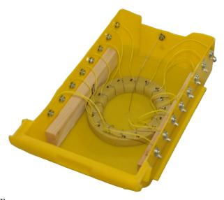
F ig. 2 Photograph of phantom built from a rubber gasket and stainless steel electrodes. The yellow dish is filled with saline.
