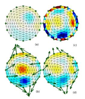
F ig. 4 Images reconstructed from experimental data. *Top Left, (a):* Reconstruction of no compression scenario. *Top Right, (c):* Reconstruction of 2-point compression assuming only conductivity change. (3-point compressions look very similar.) *Bottom:* Reconstruction of movement with 2-point (*b*) and 3-point (*d*) compressions. (Movement reconstruction with and without conductivity change resulted in similar images.) Green arrows indicate electrode movement ( $2 \times$  exaggeration).
