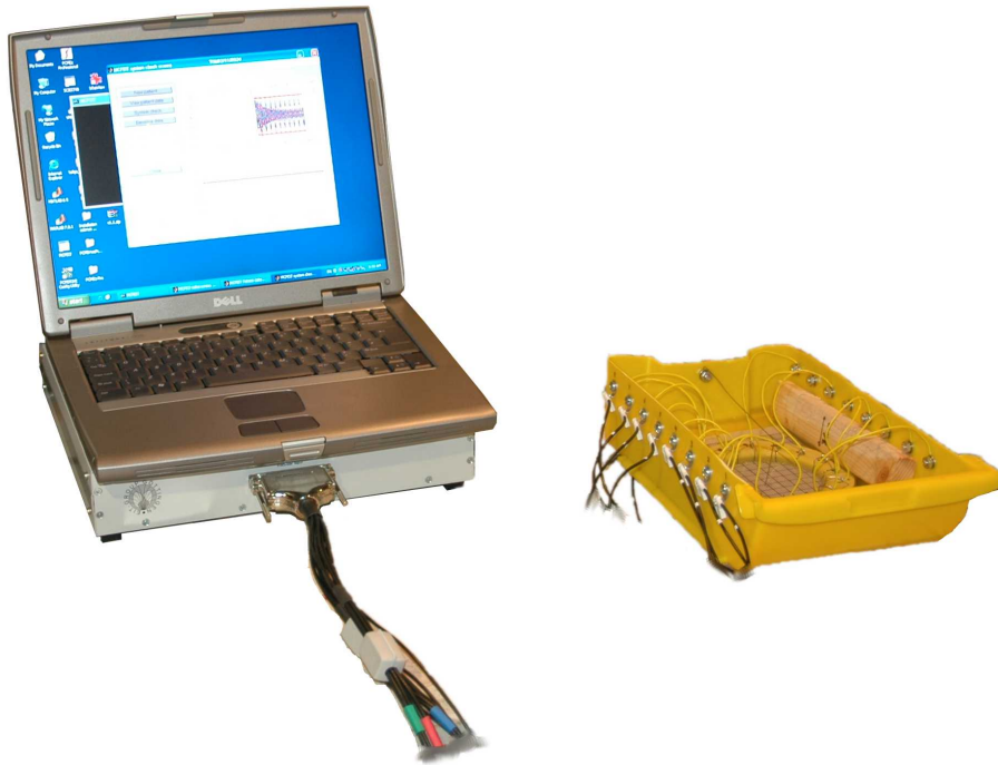
Figure 2.1: Example EIT system, photo; (left) laptop sitting on top of Goe-MF II EIT system (Viasys Healthcare, Höchberg, Germany), (right) electrode wires connecting to phantom (yellow)
