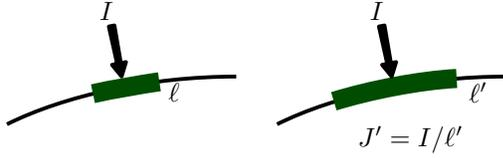
Fig. 2: Electrode current density under deformation
