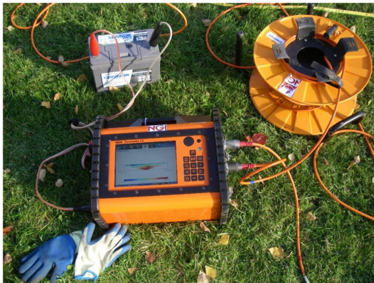
Typical ERT Survey Equipment ABEM TerrameterLS 5
