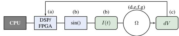
**Figure 1:** Block diagram of typical EIT hardware, consisting of (a) a storage and communication solution, typically some form of microcontroller or embedded processor and storage connected to the outside world, (b) digital frequency synthesis and modified Howland current source, (c) quadrature differential measurement, (d) analog signal chains for amplification, buffering, and filtering, (e) switching, (f) wiring, and (g) electrodes
