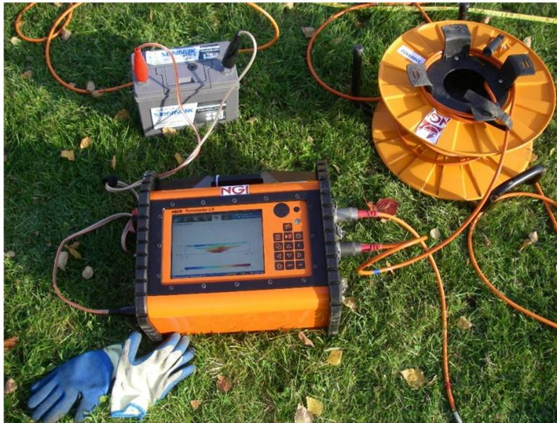
**Figure 2.1:** Example of an ERT instrument, the ABEM TerrameterLS, Image [www.ngi.no/upload/48876/TerrameterLS.jpg](http://www.ngi.no/upload/48876/TerrameterLS.jpg). The battery provides power at remote sites, and wires connect to installed electrodes.
