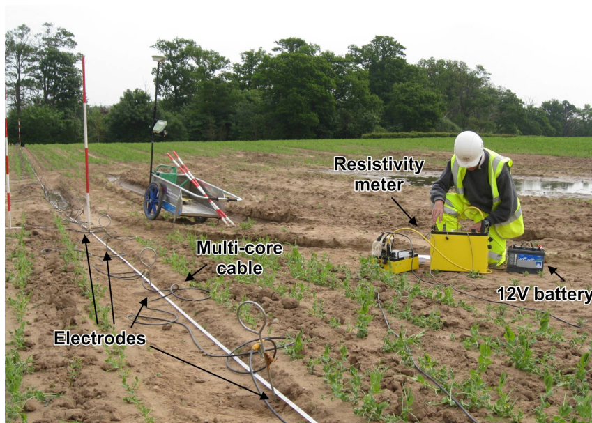
Fig 15.1: Example of an Electrical Resistivity Tomography field survey (BGS © UKRI 2019).
